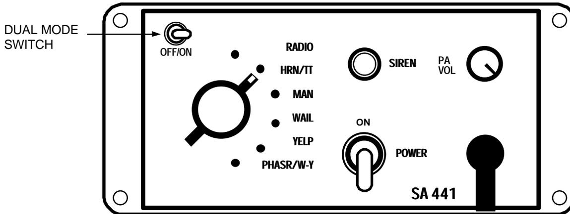
The Toggle Power Switch controls the siren power. The siren may be left on any time the vehicle is in operation. The power should be turned off when vehicle is not being used to conserve battery power.
