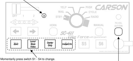
Press the OUT/DIM button momentarily to move into next section, or OUT/DIM for 3 seconds to save & exit.
