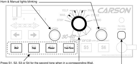
Press S1, S2, S3 or S4 for the second tone when in a corresponding Wail, Yelp or Phaser rotary switch position.
