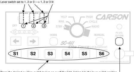
Press the desired auxiliary switch to turn on or off the light, linking it to the lever switch position. NOTE: Timed Momentary (Gun Lock Timer) programmed switches cannot be used.
