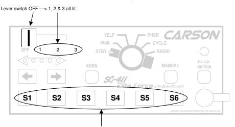
Change each switch's operation by momentarily pushing the switch.
