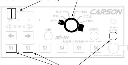
Enter the program mode by pressing and holding S1, S2 and OUT/DIM for 3 seconds.
