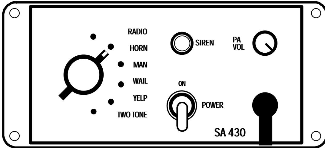
The Toggle Power Switch controls the siren power. The siren may be left on any time the vehicle is in operation. The power should be turned off when vehicle is not being used to conserve battery power.
