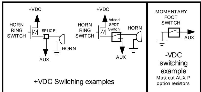
**Cutout Input Connection** - The Cutout Input turns off any siren tone output when activated, and remains off until a control is activated or changed. The adjacent diagram shows two connection examples. See the INSTALLER-SELECTABLE OPTIONS section for programming details.
