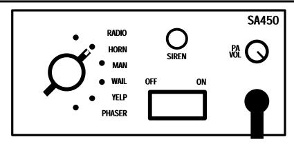
The **OFF/ON** Rocker Power Switch controls the siren power. The siren may be left on any time the vehicle is in operation. The power should be turned off when vehicle is not being used to conserve battery power.
