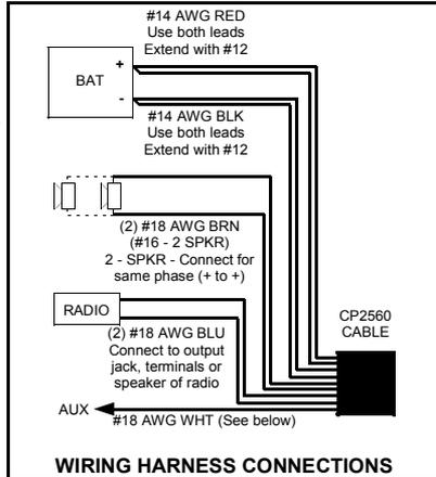
**Negative Connection (Black)** - Both leads must be used. Connect to the negative battery connector or to chassis ground.
