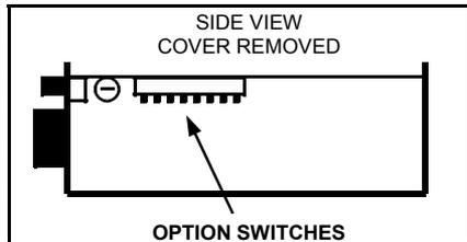
**NOTE:** Earlier models with S/N lower than 04190000 have a 5 position DIP switch and only offer the traditional auxiliary input.
